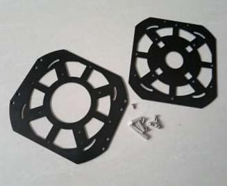
Assemble upper and bottom plate by using M3\*14.9 Alu Hex spacers X8pcs and M3\*6 srcrews X16pcs
