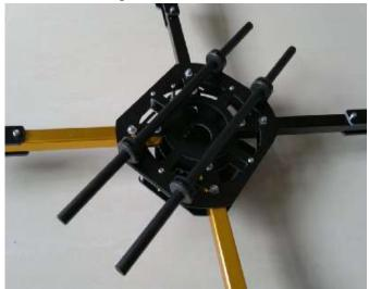
Cover rubber rings onto aluminum brock, and fix it to bottom plate alternately
