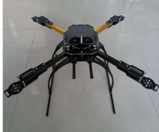
Buckle 8\*6\*35mm FG tubes onto landing gear, assembly finished.
