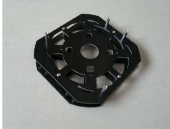
Twist 4 pcs Alu hex spacers onto both plates with M3 screws, and another 4pcs fixed one sides
