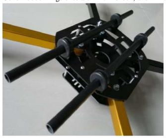
Insert the 10\*8\*30mm FG tubes and go through the rubber rings
