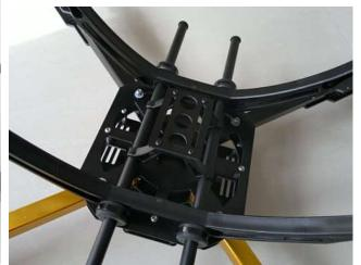
Then buckle the plastic bracket and landing gear onto 10\*8\*30mm FG tubes well
