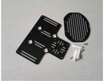
Assemble the centre board by M3\*25 Nylon spacers and M3\*6 screws, then fix the cover on it
