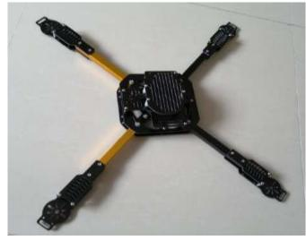
Then fix the centre comtrol board onto main frame plates
