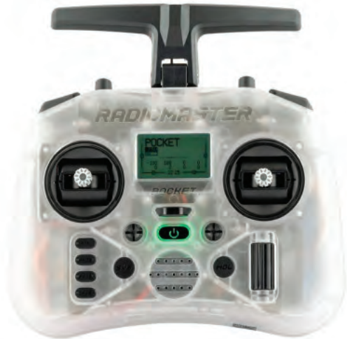
RADIOMASTER (Transparent) Pocket CC2500 FCC 2.4GHz Compact 16ch Transmitter w/Open-Source Edge TX Firmware
