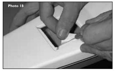
There are two access hatches. One in the front in case you have to put your batteries in the nose of the plane for proper balance, and one in the rear for installation and maintenance of the rudder and elevator linkage.
