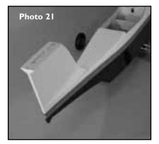
On the top of the fuselage, about 10" from the rear, there is a pre-drilled hole for the elevator's outer nyrod to exit. Cut away the covering material from this hole. By the same token, there is a slot in the left side of the fuselage, about 3" from the rear. Cut away the covering from this slot.
