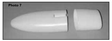
The engine pod is blowmolded plastic. To cut this material, score a few times with a sharp utility knife. Once a cut-out is made, you can whittle away the rest or use a Dremel tool with a sanding drum.. Work carefully. It is easy to cut too much away; it is also easy to cut yourself.
