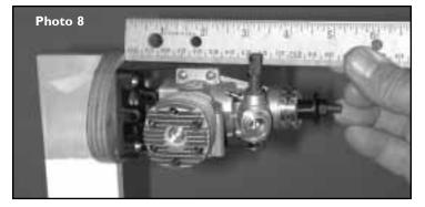
Position your engine on the engine mount (note that the mount's beam width is adjustable to accommodate your engine). Locate the engine on the mount so the front of the prop's thrust washer is  $4 \ 1/4$ " from the front surface of the firewall. Double check that this set-up gives you 1/8"-1/4" of spinner clearance from the front of the engine pod. Mark then drill pilot holes using a 3/32" bit. Mount your engine using the four M3 X 15mm screws.
