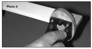
Secure the engine mount assembly on the firewall using the four screws and blind nuts furnished. (Normally, the engine is side-mounted with the cylinder head on the right.)
