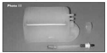
Assemble the fuel tank as shown. The fuel tank is housed in the rear engine pod and held in place with lightly wrapped foam rubber.
