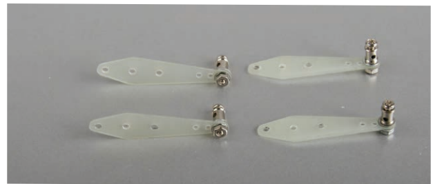
19. Install pushrod adjuster into the hole of servo arm extension.
