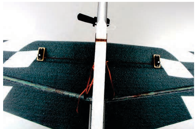
12. And fix the servos onto the plywood servo mount with included screws. Use knife to cut slots on wing, then embed aileron servo leads as picture shown.
