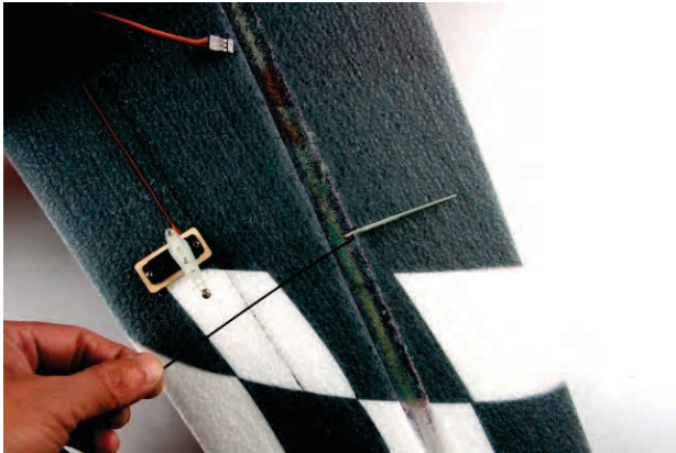
23. Connect Z bend into the hole of control horn.
