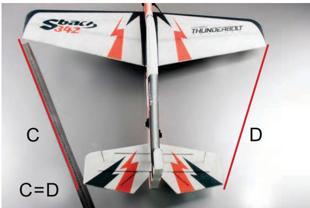
13. Insert elevator into the slot of fuselage. Make sure C=D (refer to the picture).
