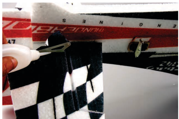
22. Cut a slot on control surface along a ruler, and insert control horn into this slot, then use CA to fix. The same operation on aileron, elevator & rudder control horns.
