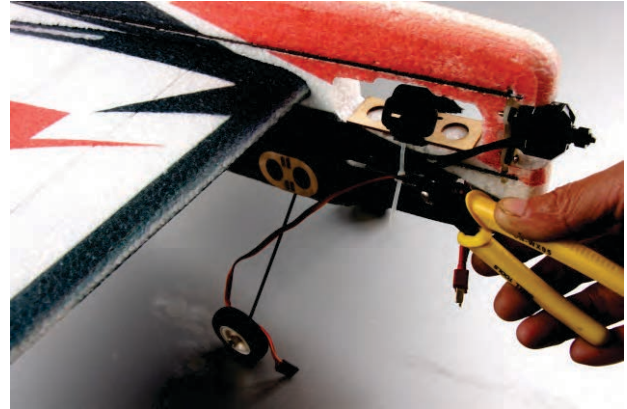
33. After test, put the receiver into the receiver slot(see picture).
