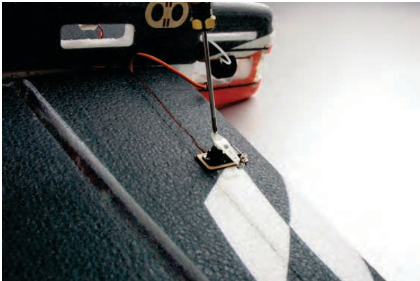
17. Fix trimmed servo arm with included screw.
