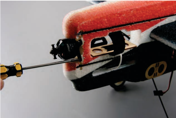
29. Use included screws to fix the motor onto the motor mount.
