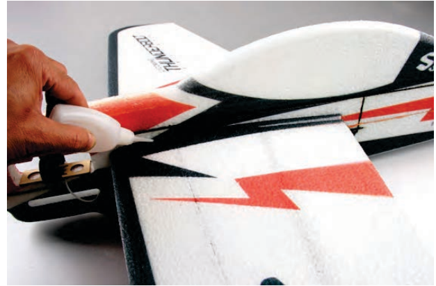
9. Drop some glue on the joints of fuselage and wing to fix (both upside and downside).
