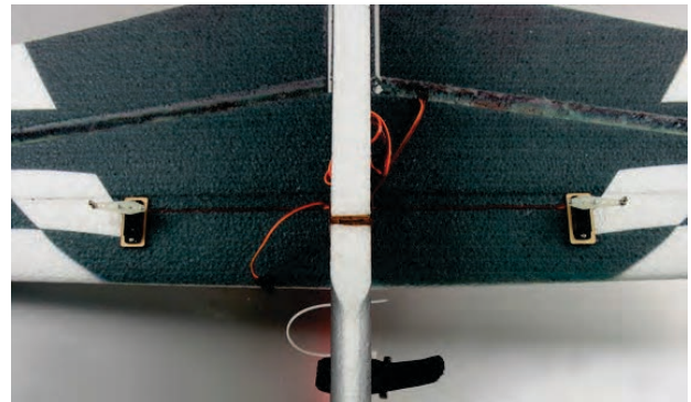
20. Fix servo arm extension on servo arm with 2pcs 2*4mm self tapping screws.
