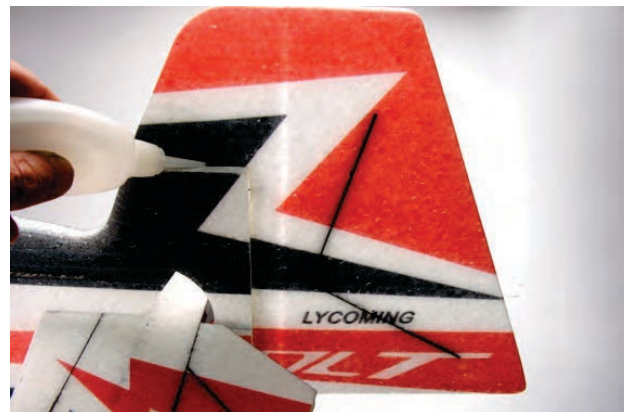
15. Use CA to fix the rudder.
