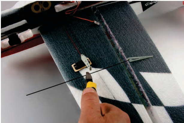
24. Reserve proper length of Z bend, then cut off additional part that you don't need.
