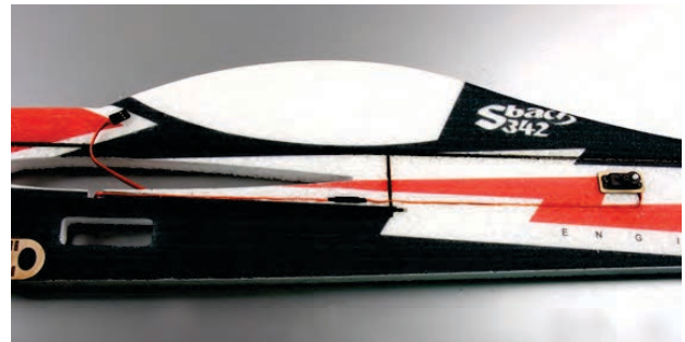
6. Embed servo leads into the slot.
