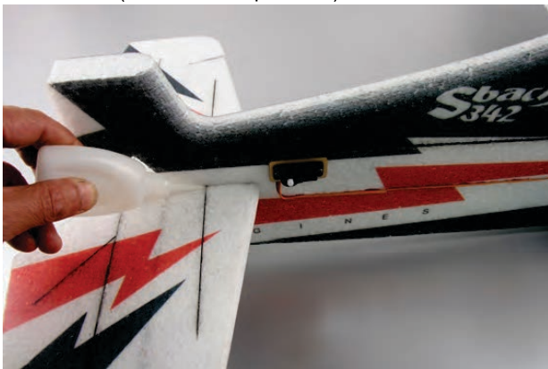
14. Drop some glue on the joints of elevator and fuselage to fix.
