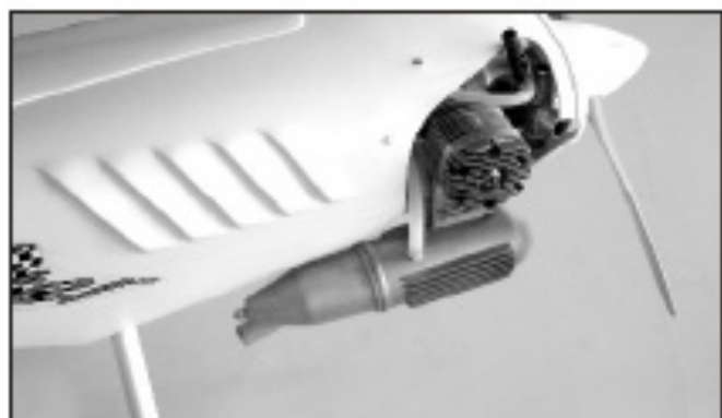
53. Connect the fuel tubes properly to the muffler and the carburetor.
