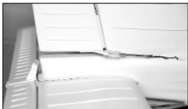
55. Locate the threaded end w/hole, thread it into the clevis at least 6mm then loop the other end of cable as you did on Z-bend end. Snap on the clevis to the rudder control horn then adjust the tension and make the circle as small as possible. Make sure both cables are equal and the brass tube will not contact the exit hole when servo works. Once satisfied, clamp the brass tube. You can adjust the tension by threading in or out of the clevis.
