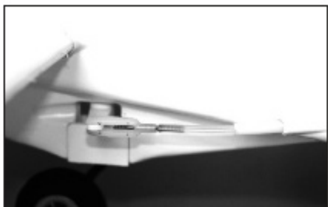
58. The guide tube will come out from a fairing with inner tube inside at the bottom tail where need to be drilled for a hole. Thread the clevis and snap the clevis on the steering arm while rudder servo is in neutral position. Apply a silicon ring to the clevis.
