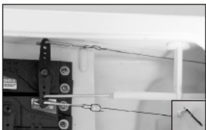
57. Enlarge the hole of the guide tube retainer with 5mm(13/64") drill bit. Install the guide tube retainer and glue the guide tube in place. Note the servo horn need to be cut if you use the long one as it may contact the elevator servo horn. The Z-bend end of tail wheel pushrod is installed at the left side and second hole of the servo horn. You may remove the servo horn from the servo for easy installation.
