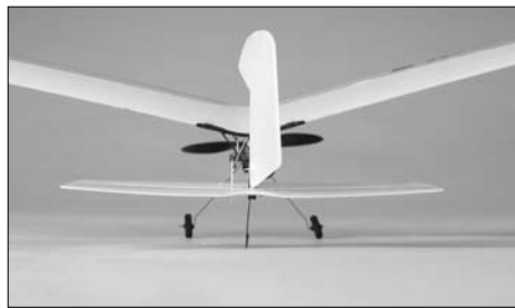
Shown with aileron stick pushed to the right.
