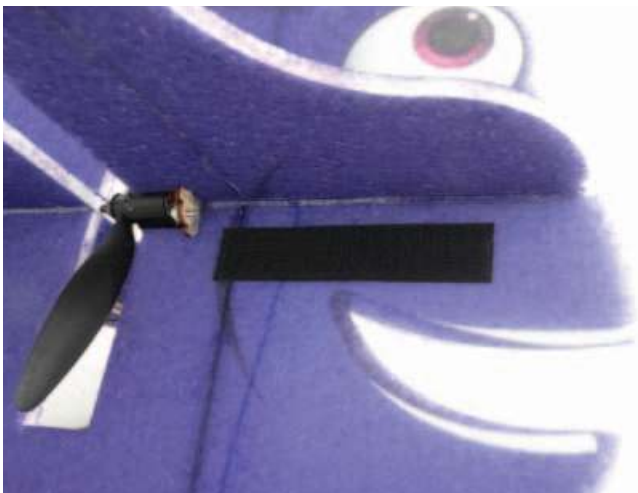
Put hook and loop tape on fuselage using foam glue behind ESC.
