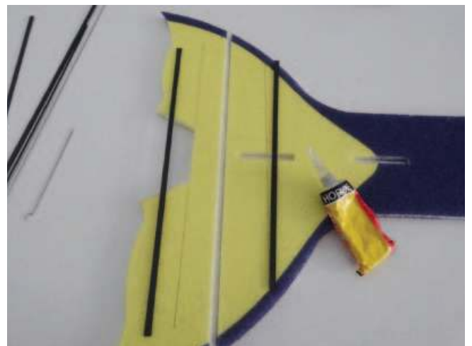
Install carbon strip on horizontal tail using foam glue or No.502 glue. Then wait glue dried.
