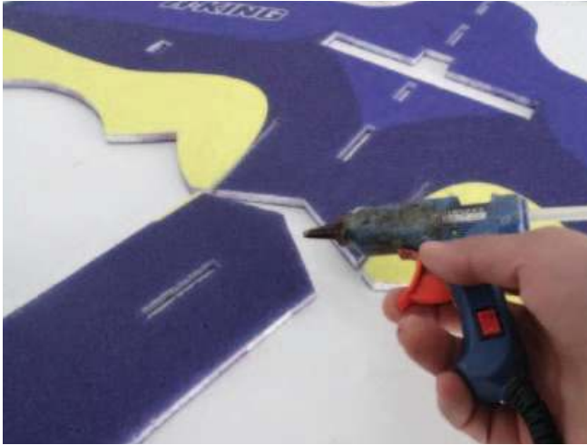
Glue the 2 pcs horizontal fuselages using hot glue sticks.
