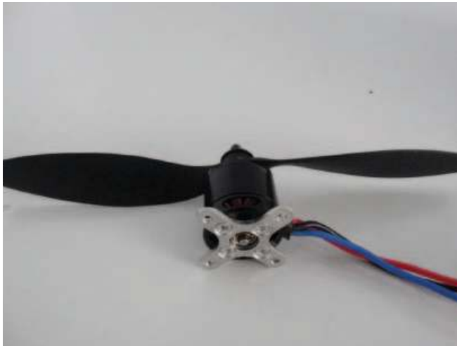
Assemble motor on the metal cross using screws. Assemble prop on motor. Notice the prop's direction.
